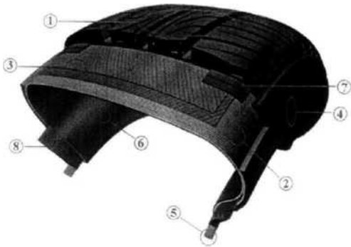
1. Tread 2. Carcass 3. Belt 4. Sidewall 5. Bead 6. Inner liner 7. Capply 8. Apex
